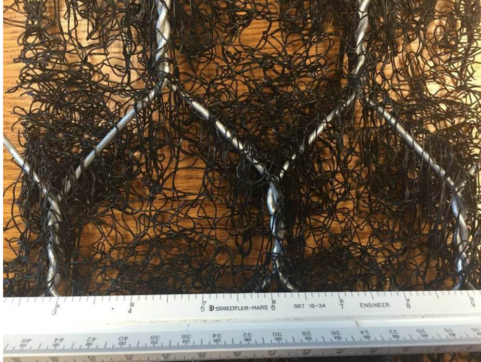
Figure 7-34. Example of polypropylene erosion mat woven with mesh
