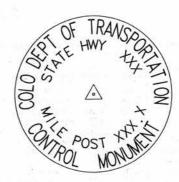
CM-MP - Control Monuments were set by CDDT. They were CDDT type 2 monuments, a  $3-1/4^{\prime}$  dia. aluminum control monument cap (as shown) on a 3' X  $3/4^{\prime}$  dia. finned aluminum security rod on a 3' X  $3/4^{\prime}$  dia. smooth duminum rod.
