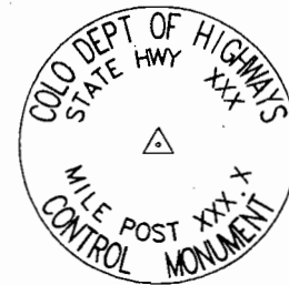
Typical Control Monument Cap Not to Scale
