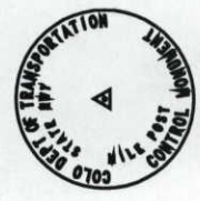
Typical Control Monument Cap Here to Scale
