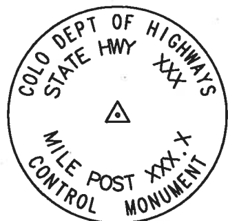
Typical Control Monument Cap Not to Scale
