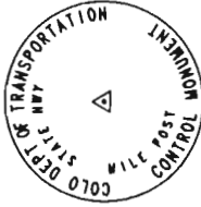
Typical Control Monument Cap Not to Scale
