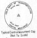
CP - Control Point Monuments set by CDDT. All Control Point Monuments unless otherwise noted are CDDT Type 2 monuments, which consist of a 3-1/4" dia. aluminum control monument cap (as shown) on a 3'  $\times 3/4$ " dia. finned aluminum security rod and 3'  $\times 3/4$ " dia. smooth aluminum rod assembly.
