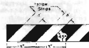
DETAIL OF RAIL AND WING STRIPING
