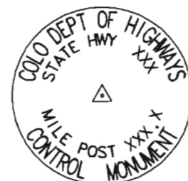
Typical Control Monument Cap Not to Scale
