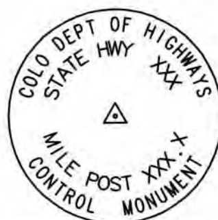
Typical Control Monument Cap Not to Scale
