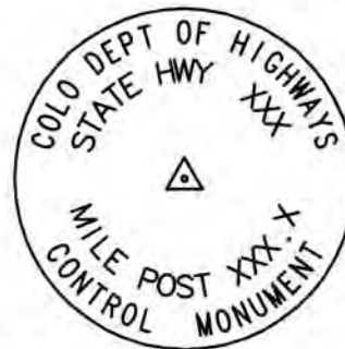
Typical Control Monument Cap Not to Scale
