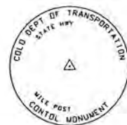
Typical Control Monument Cap Not to Scale
