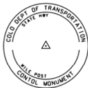
Typical Control Monument Cap Not to Scale
