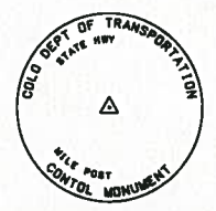
Typical Control Monument Cap Not to Scale
