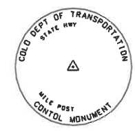
Typical Control Monument Cap Not to Scale
