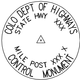
Typical Control Mounment Cap Not to Scale
