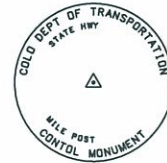
Typical Control Monument Cap Not to Scale
