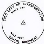
Typical Control Monument Cap Not to Scale
