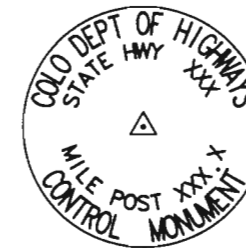
Typical Control Monument Cap Not to Scale
