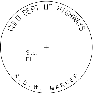
Fnd. 3/4" Brass Cap set in 6" dia. concrete Pt. Nos. 1015 & 1018
