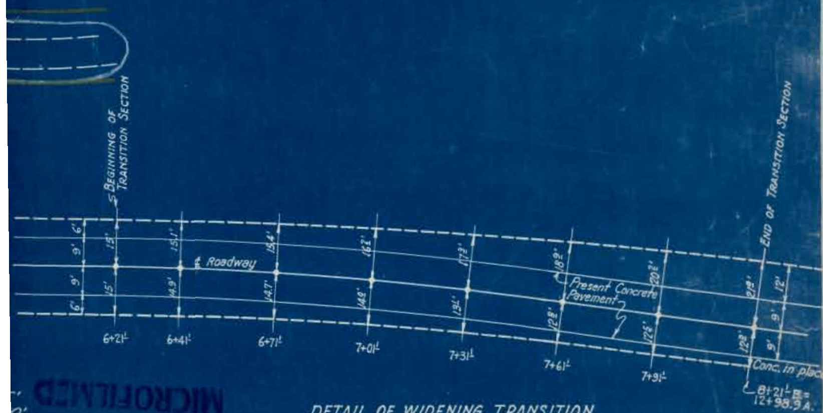
DETAIL OF WIDENING TRANSITION STA. 6+21 TO 8+21
