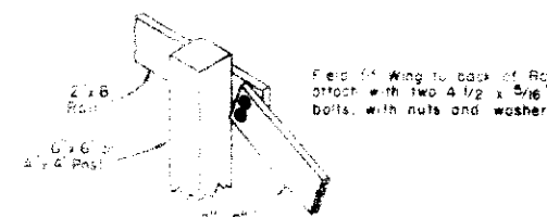
REAR VIEW OF BARRICADE SHOWING WING ATTACHED (See Note No. 9)
