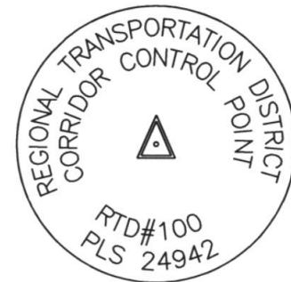
Typical Control Monument Cap Not to Scale
