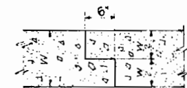
HALF-LAP CONSTRUCTION JOINT
