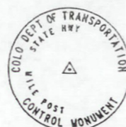
Typical Control Monument Cap Not to Scale
