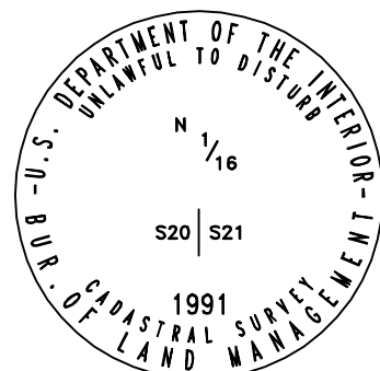
Found 3 1/2" Aluminum cap on 3" iron pipe 1.0' above ground Point # 174
