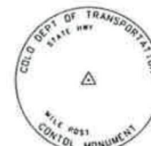
Typical Control Monument Cap Not to Scale
