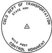
Typical Control Monument Cap Not to Scale
