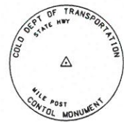
Typical Control Monument Cap Not to Scale
