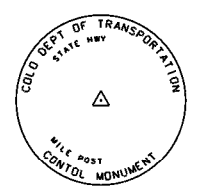
Typical Control Monument Cap Not to Scale
