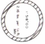
BRACE RAIL & TOP RAIL
